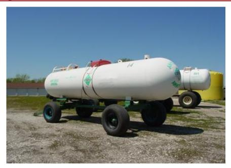
Catastrophic results can occur when unauthorized repairs are performed on high pressure vessels transporting anhydrous ammonia (NH3). An improper weld on a nurse tank was a factor in a nurse tank failure that occurred on April 15, 2003 near Calamus, IA. resulting in one fatality and one serious injury. This is a stark reminder of the serious consequences that can occur as a result of a nurse tank failure.
