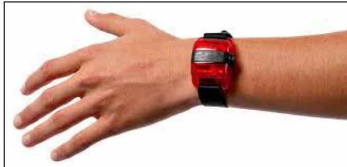
Figure 3. Image. Wrist Actigraph wGT3X-BT, produced by ActiGraph Company.
