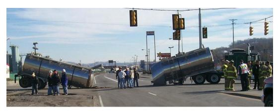
About 11:36 a.m. on January 5, 2002, a tractor pulling a cargo tank semitrailer departed the plant entrance and the trailer catastrophically failed. This failure occurred in the void area between the first and second tank, and the trailer broke into two pieces.
